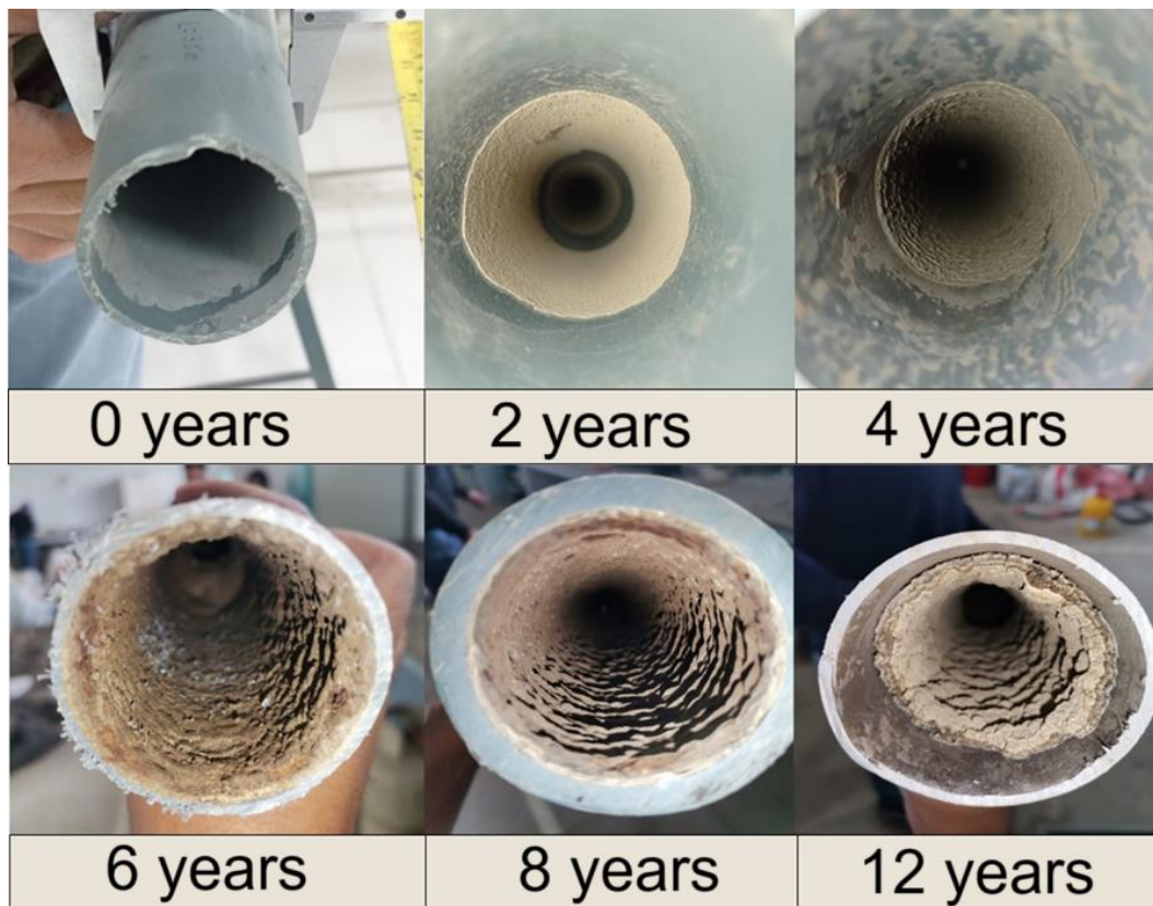
Figure 4: Variation of roughness in the study pipes over time.
