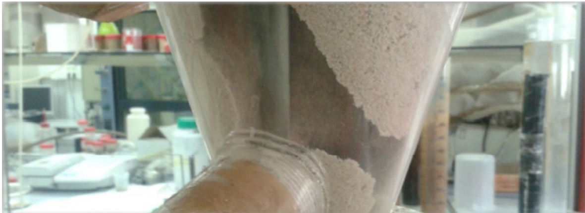
Figure 3: Image of the cavity open when the wet sand is stuck on the walls of the contactor ( x_L = 10\% d.b.)
