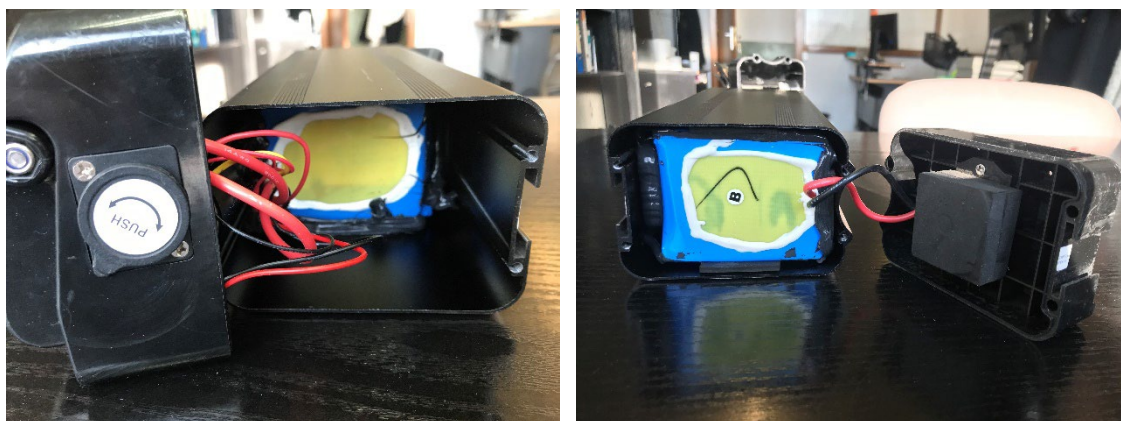
Figure 2: Pictures of the casing and cells inside the battery pack
