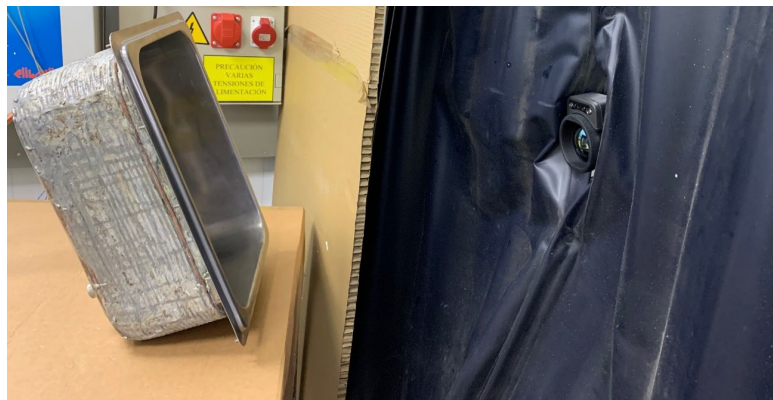
Figure 5: Set up of the infrared thermography inspections.
