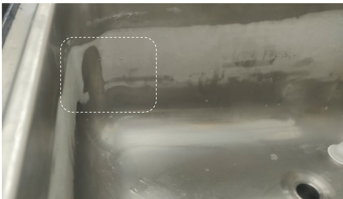
Figure 7: Stainless steel container in normal operation for storing ice-cream. Certain zones presenting uneven cooling can be observed.
