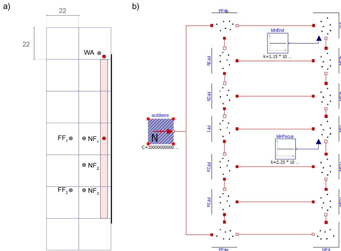
The Modelica model can be seen in Figure 3 b), where there is a room element for each cell, the two constant emission factors with Standard Modelica Library blocks and the constant outdoors concentration with the “FixedConcentration” element.
