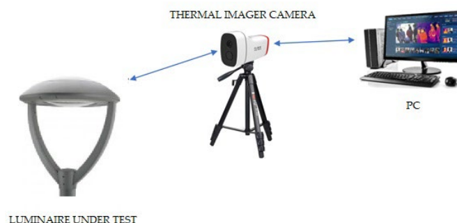
Figure 1: Experimental Set-up for the measurement of thermal dissipation. Source: Own elaboration
