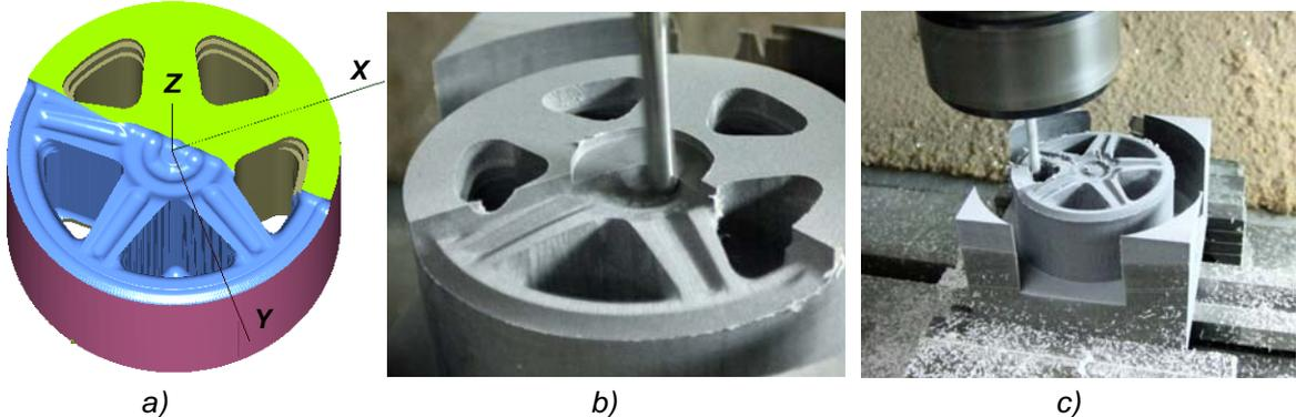
Figure 12. a) Simulation of stage 7; b) and c) Different stages of wheel and rim machining.
