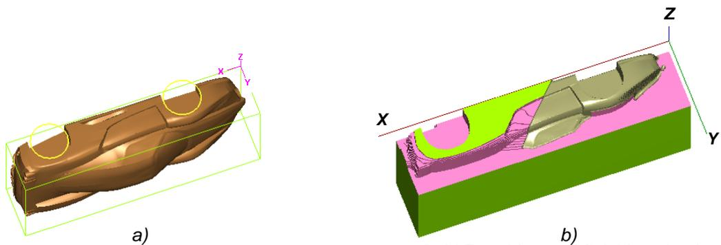
Figure 8. a) Model orientation to programme the stage 3; b) Roughing and finishing simulation.
