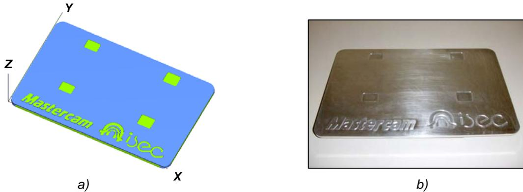
Figure 13. a) Machining simulation of the base; b) Aluminium base after polishing.
