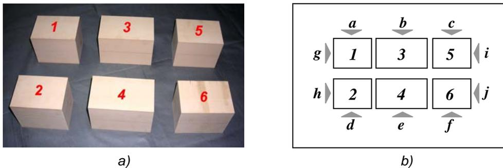
Figure 2. a) Initial polyurethane blocks where the milling is performed; b) Schematic figure of blocks with numeration and face's designation.
