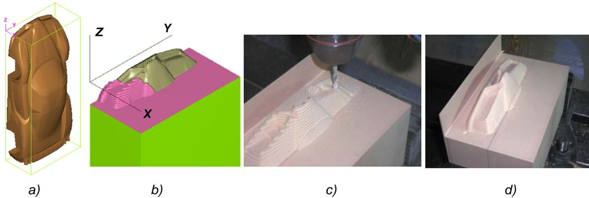
Figure 6. a) Model orientation to programme the stage 1; b) Roughing and finishing simulation; c) Front part during roughing cycle; d) Front part after finishing cycle.
