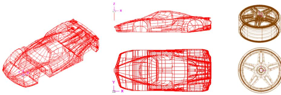
Figure 1. Different views of Enzo Ferrari model obtained in CAD software (IGES format).
