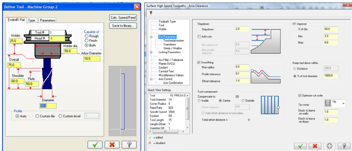
Figure 4. Tool and cut parameters selected for a specific roughing toolpath.
