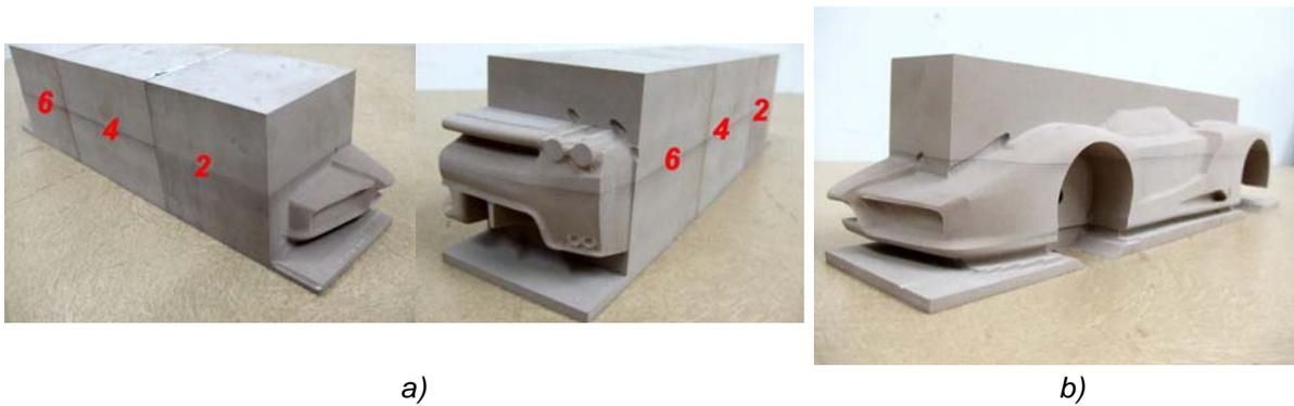
Figure 9. a) Two different views of blocks 2, 4 and 6 before being submitted to the milling process; b) Left part after to be submitted to the stage 3.
