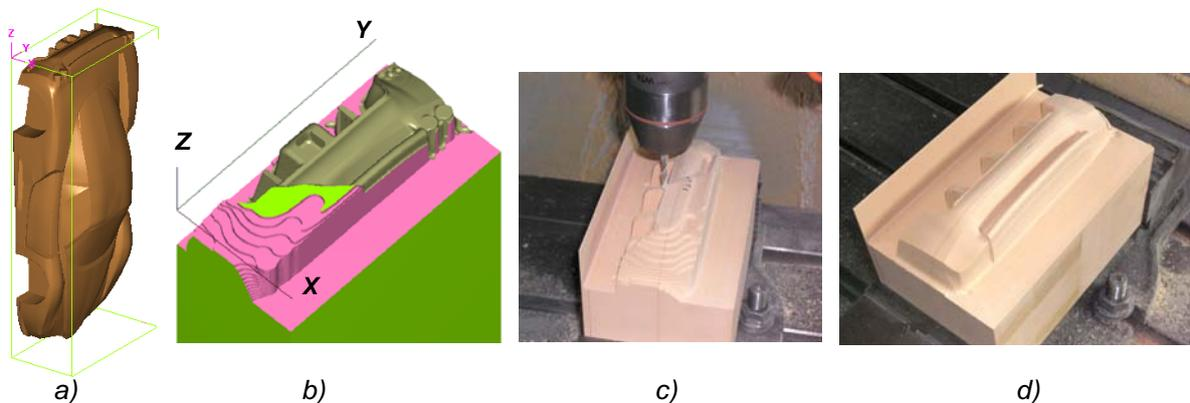
Figure 7. a) Model orientation to programme the stage 2; b) Roughing and finishing simulation; c) Rear part during roughing cycle; d) Rear part after finishing cycle.
