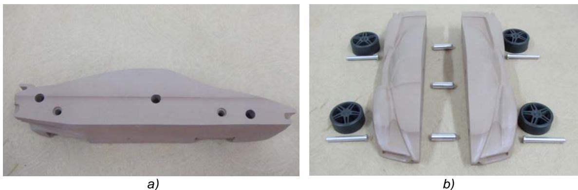
Figure 14. a) Holes opened in machined parts; b) Parts of Enzo Ferrari before assembly.
