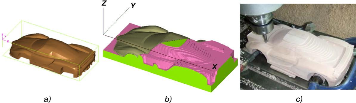
Figure 11. a) Model orientation to programme the stage 6; b) Roughing and finishing simulation; c) Top part during roughing cycle.
