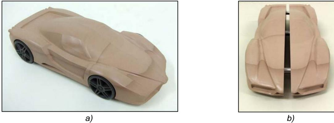
Figure 15. a) Car after assembly; b) Detachment of the car in 2 parts.
