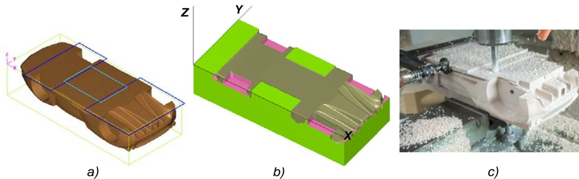
Figure 10. a) Model orientation on stage 5; b) Simulation of stage 5; c) Bottom part machining.
