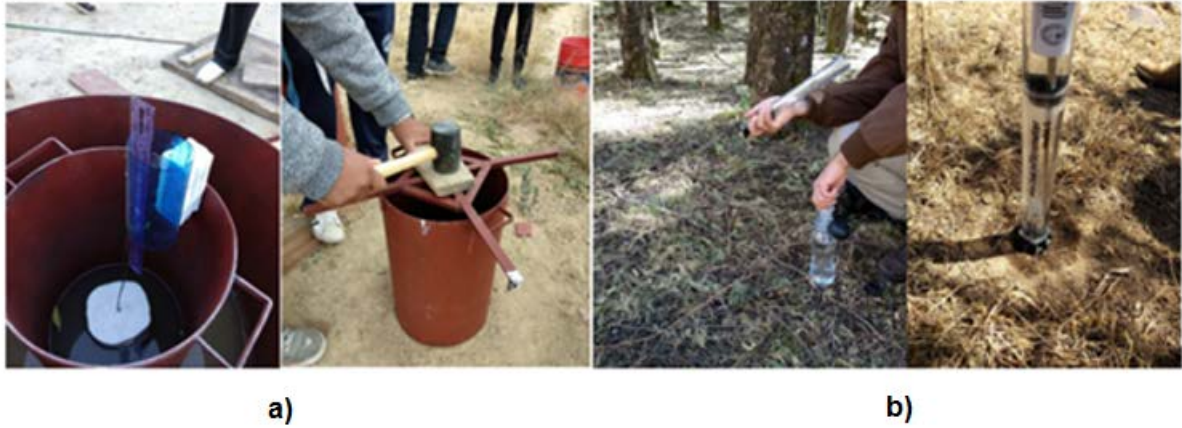
Figure 5: Installation and measurement: double ring (a) and Minidisc Infiltrometer (b)
