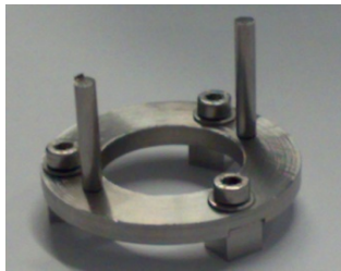
Figure 12: FRICTORQ III: The redesigned contact body, with three small square shaped pads
