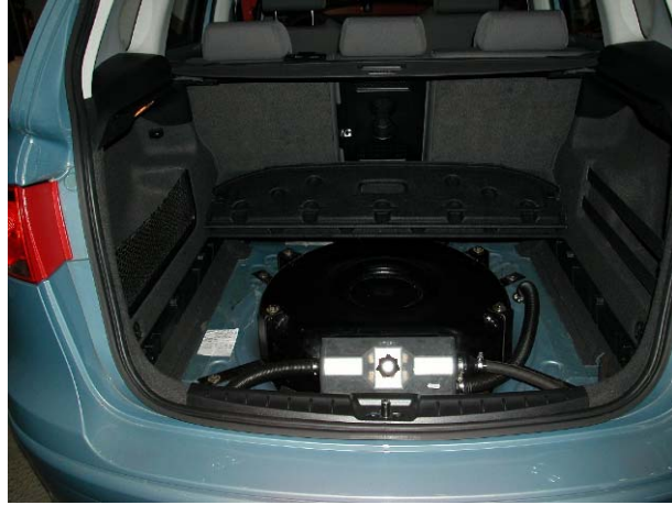
Figure 2. LPG tank and fuel lines housed beneath the luggage floor
