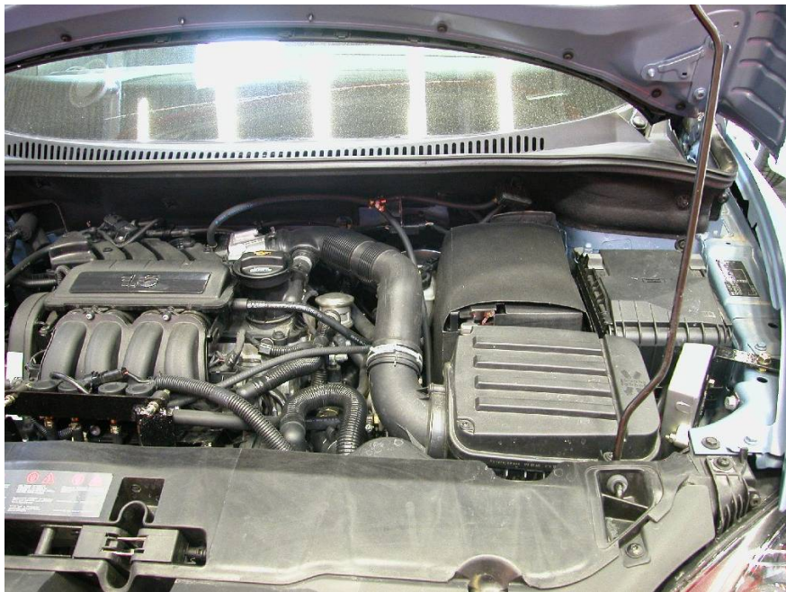
Figure 6. LPG ECU located on left-hand side of engine bay
