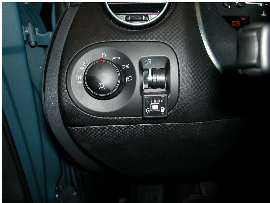
Figure 8 Gas switch and level indicator located in general light switch A2 Engine power and torque curves Petrol mode / LPG mode
