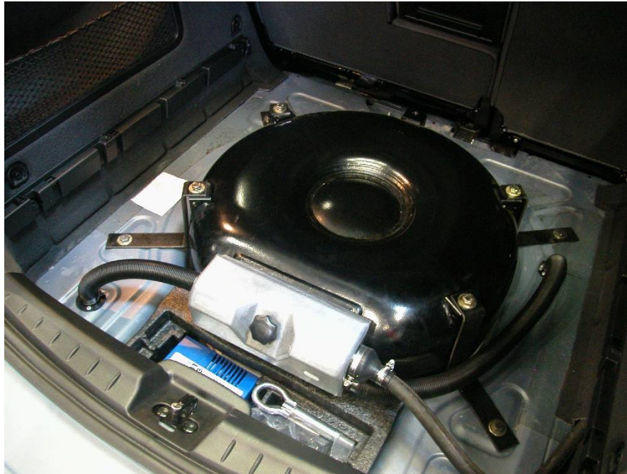
Figure 7. Tyre-fit set and tool kit located in recess behind LPG tank
