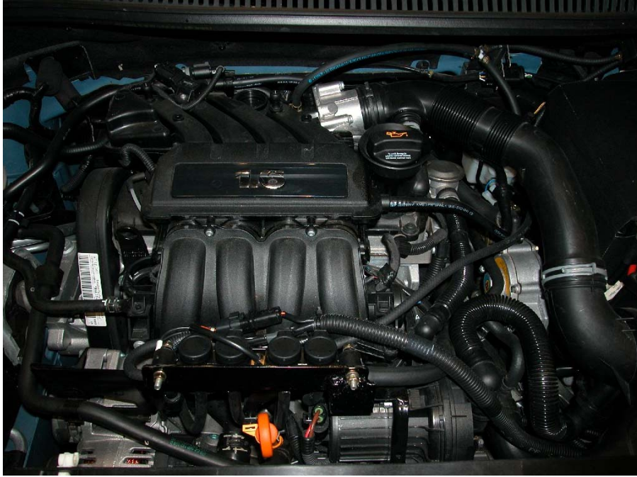
Figure 5. General view of engine bay with LPG installation
