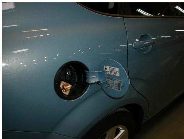
Figure 4. Petrol and LPG fillers located behind the same cover
